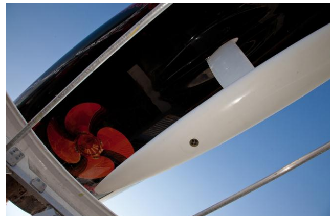
Nortek DVL installed in keel of Puma's Mar Mostro. Photo courtesy of PUMA Ocean Racing Team, Alicante.
