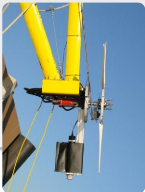
Aquadopp Profiler Mounted on UNH Test Turbine
