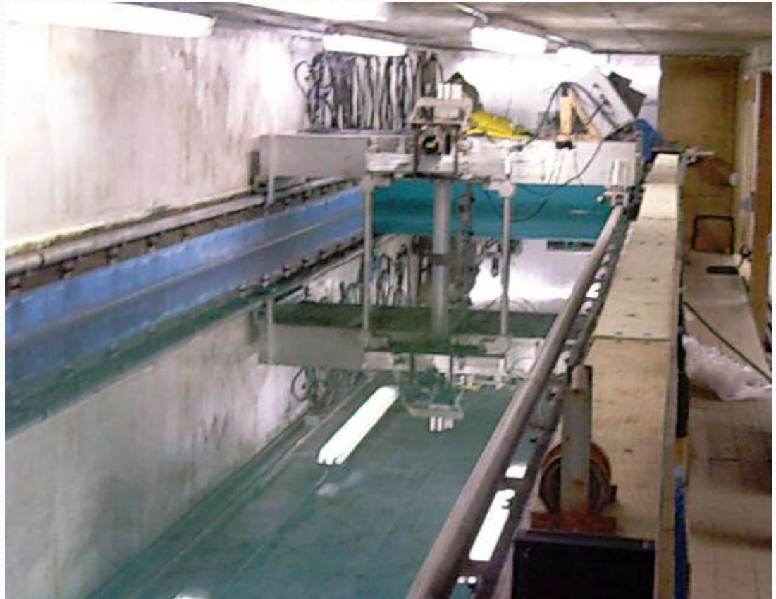
Cross-Flow Turbine Test Bed in University of Maine Tow Tank
