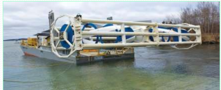
ORPC's Cross Flow Tidal Turbine to be Tested in Eastport Maine.
