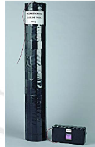
Same operating life with smaller size for use in GPSlice buoys. Oceantronics' original battery pack (left) used 380 alkaline D cells (54 kg). The new battery pack (right) uses 32 lithium thionyl chloride D cells and four hybrid layered capacitors (3.2 kg).
