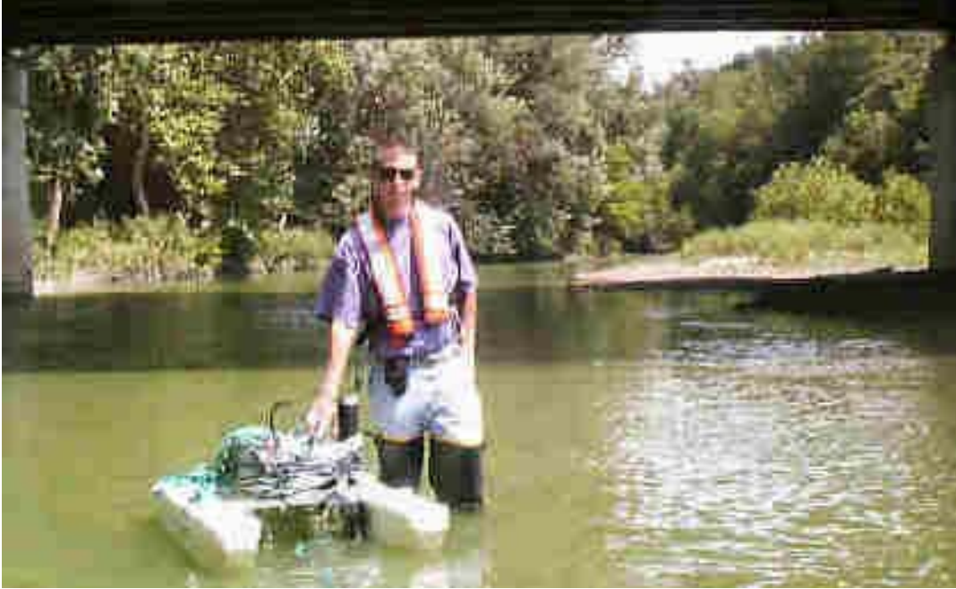
Figure 2. USGS Hydrologist Scott Morlock holds the Aquadopp Profiler on station during a measurement. The profiler was mounted on a tethered boat designed for river discharge measurement using Doppler profilers. Data were telemetered to a PC on the riverbank.
